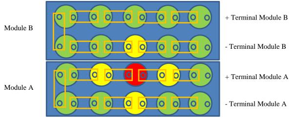
All dummy cells (green) are short circuited between its cell terminals to allow charging over the + and – terminals of the modules.
