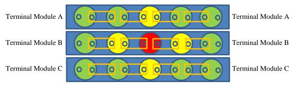
All dummy cells (green) are short circuited between its cell terminals to allow charging over the + and – terminals of the modules.
