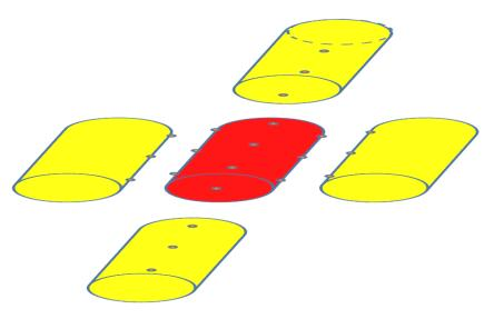
On a cylindrical cell to be treated (red) there shall be mounted 13 thermocouples to get a temperature distribution of the surface temperature of the cell. 12 thermocouples on the cylindrical surface, 4 mounted around the diameter and three of such "rings" distributed over the longitudinal axis. The thermocouple 13 will be located where the venting area is located.
