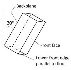
Figure 1. Orientation of DUT before release in drop test. The front face is the face facing the user during normal operation.
